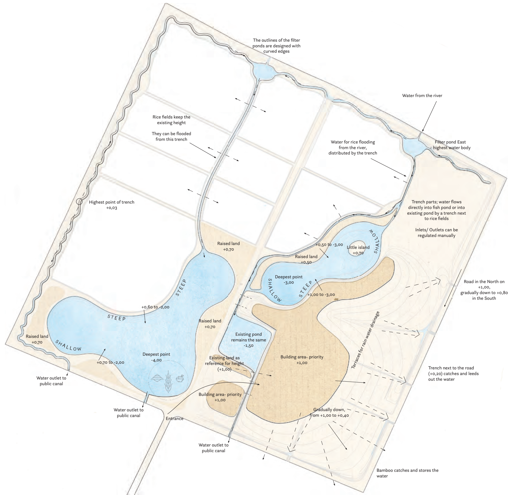
concept earth works, water management and flow
